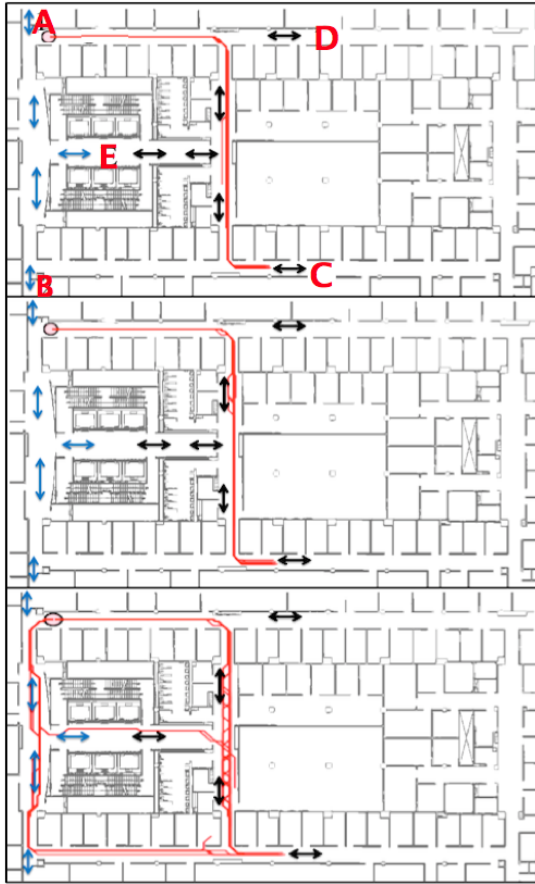
Figure 8: All plans generated by A* (top), CSA* (middle) and Risk-A* (bottom) to reach the (circled) 4th target. Arrows and numeric labels describe crowd behavior. (See text.)
