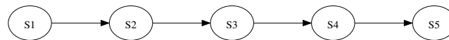
Figure 1.5: A data dependence graph exhibiting no parallelism. The tasks must be performed one after the other, from left to right.
