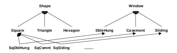
Figure 3 Three Level Multiple Inheritance
