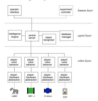
Figure 2: System architecture
